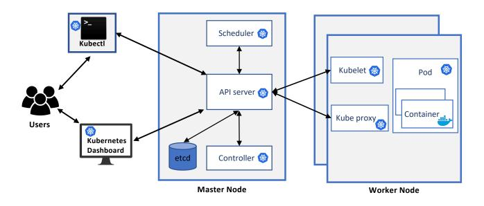
Fig. 1: A brief overview of Kubernetes. Kubernetes users interact with the installation using the Kubernetes dashboard and 'kubectl'. The purpose of master node is to maintain the desired cluster state and manage worker nodes. Worker nodes are used to run containerized applications inside the pod.
